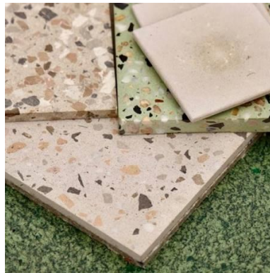
Figure 35. Ceramic products remanufactured from local waste streams.
