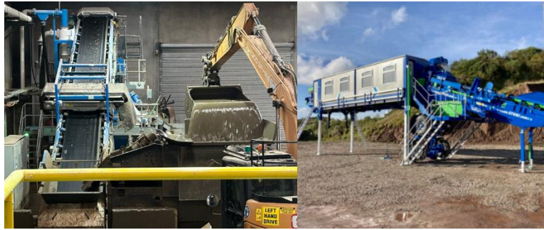
Figure 34. Wet processing of soil waste (left) (CDE Group) (CDE Group, 2024) and mobile picking stations (right) (Waste Initiatives)
