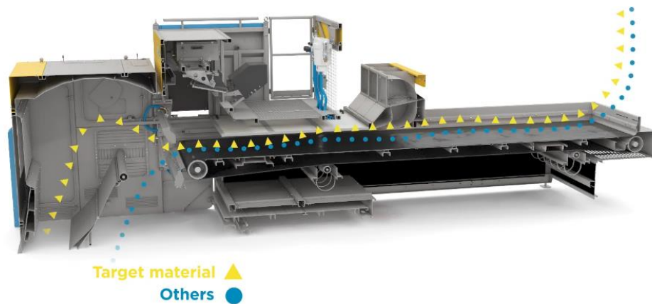
Figure 16 - Diagram of Near-infrared (NIR) sorter (Pellenc St)
