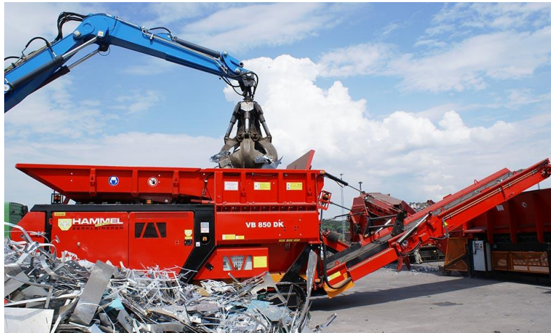
Figure 20 - Slow-speed shredder for heavy duty applications (CSS Equipment)
