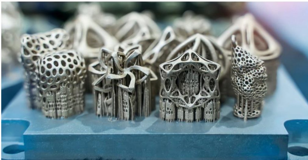
Figure 28 - Examples of metal products made from Additive Manufacturing (Continuum Powders)
