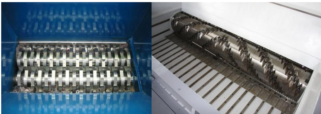
Figure 19 - Shredders: single shaft (left) (Fordura), twin shaft (right) (Brentwood Recycling Systems)
