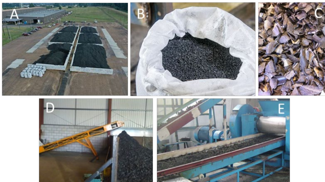
Figure 4 Images showing storage and handling of crumbed/shredded tyres, including (A) processed EOL tyre stockpiles, open to ambient environment; (B) bagged EOL tyre crumbs; (C) coarse shredded tyres, stored in a stockpile; (D and E) use of a conveyor to move material to a stockpile housed inside a processing facility.
