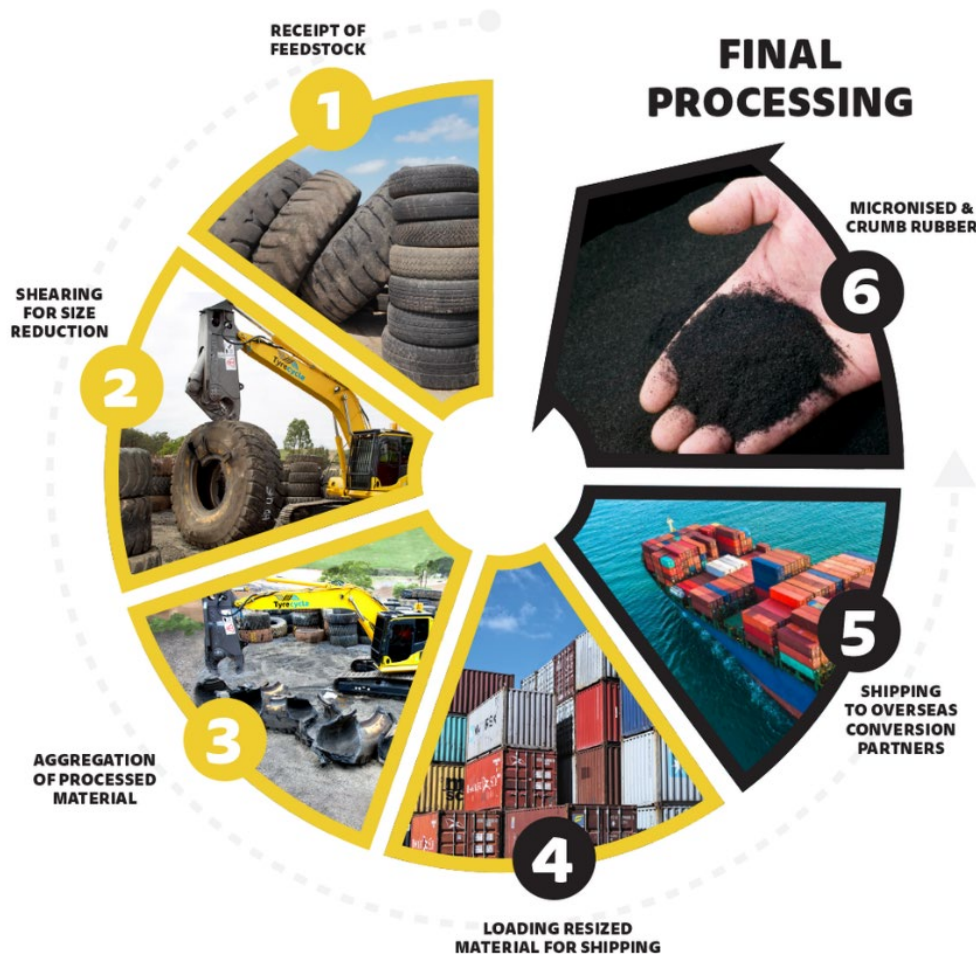
Figure 18. Tyrecycle OTR tyre recovery process model (Reused with permission from Tyrecycle).
